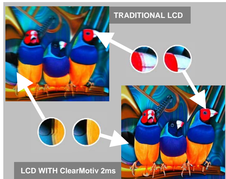
Figure 6: Traditional 8ms LCD vs ClearMotiv 2ms (10 pixels per frame)
